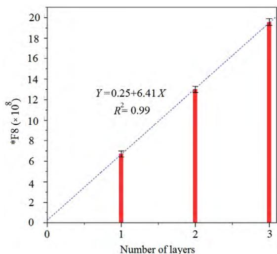
Figure 3. Dependence of \*F8 tally on the number of active layers in the MD-55-2 radiochromic film. The film was positioned at 10 cm depth of a water phantom
