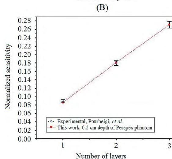
Figure 5. Normalized sensitivity versus the number of layers of the MD-55-2 film. Monte Carlo results were compared with the results of Pourbeigi, *et al.* (A): For 12 cm x 12 cm film. (B): For 4 cm x 4 cm film
