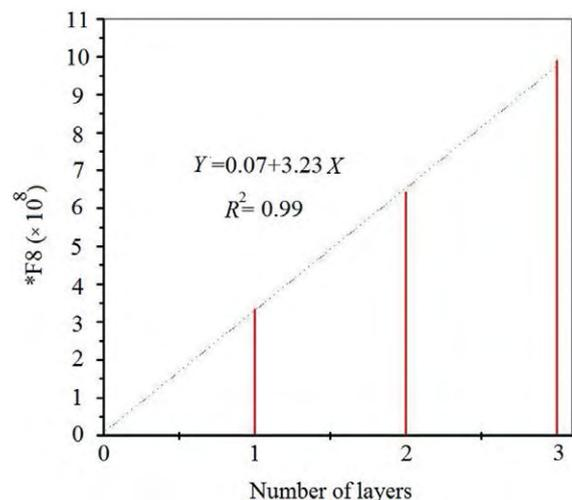
Figure 4. Variation of \*F8 tally versus the number of active layers of the MD-55-2 film positioned in 0.5 cm depth of a Perspex phantom
