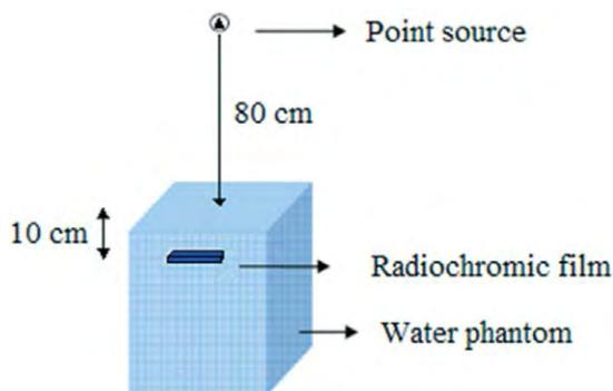
**Figure 1. Geometry of the simulation illustrating position of the source, phantom and radiochromic film**
